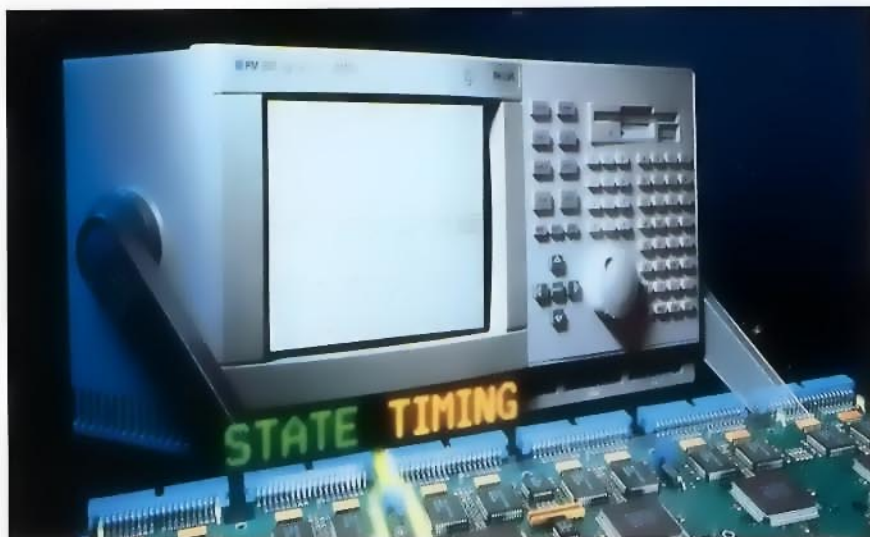
The Philips PM 3580 logic analyzer from Fluke speeds logic analysis by reducing state and timing measurements to one probe connection.
